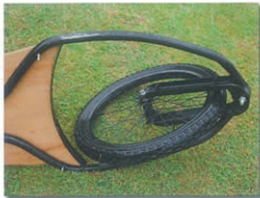
Front wheel pivots on swing arm.
