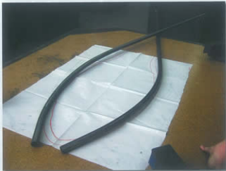
Tube checked against the full-size drawing.
