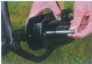
Swing arm attaches through bearing.
