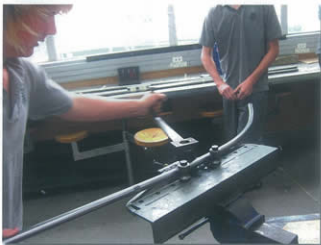
Bending the steel tube.
