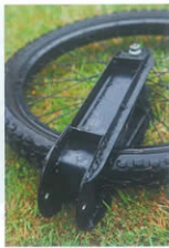
Kyle reinforced the swing arm with extra welding.
