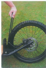
Braking system pulls on wire.
