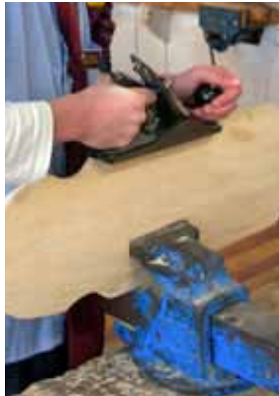
Planing is followed by shaping using a spokeshave for finer details
