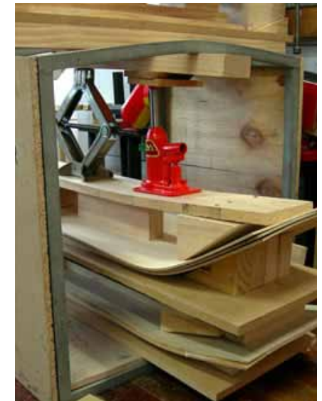
Alexia’s highly innovative, easily affordable solution to the problem of bending the wood in a press to shape the curvature of the board – use a bottle-jack!
