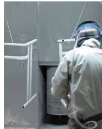
Powder coating is done at the Furnware factory – a dry powder is sprayed alongside the unit and is attracted on to the surfaces using electrostatic forces.
