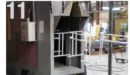
11 In powder coating, a dry powder is sprayed alongside the unit and is attracted on to the surfaces using electrostatic forces.
