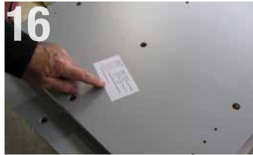
16 Each panel is labelled when done – with job number, part name, etc – to facilitate assembly.
