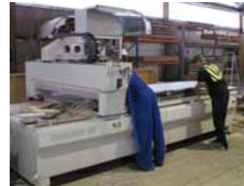
Cutting and drilling of the panels is done automatically by computer-controlled cutters on a large flat-bed machine.
