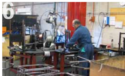
6 Furnware has two welding robots Pat: "Robotic welding gives consistently high quality welds – you don't get the little bits and pieces that you tend to have with a hand welded product."
