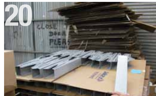
20 The side storage unit is assembled here – the part shown screws onto the desk. The metal is laser cut and pressed into shape by a subcontractor and is powder coated at the Furnware factory.
