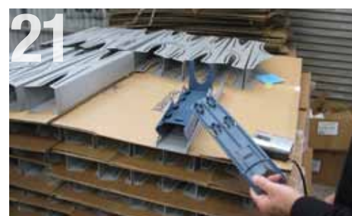
21 The plastic slider mechanisms are then fitted into the metal bracket.
