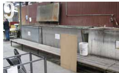
9 Before powder coating, the metal has to be completely cleaned or else the powder coat doesn't bond properly, so the welded units are cleaned in a three-step immersion process.
