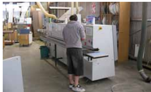
17 The edge banding machine runs an PVC edge around the cut MDF panels. It applies hot melt to the tape as it is rolled on to the edges, and trims the tape. Pat: "It's a New Zealand design, computer-controlled and very reliable."
