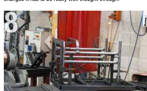
7 The pieces to be welded for a desk being set up in a jig. Pat: "Making a jig is quite an involved process, so if something changes it has to be really well thought through."
