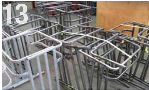
13 After baking the units have an anti-graffiti glaze put on them.
