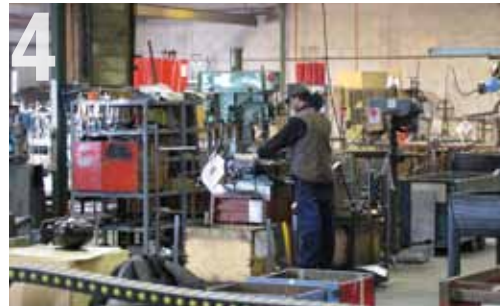
4 Holes for various components are punched or drilled in the metal.
