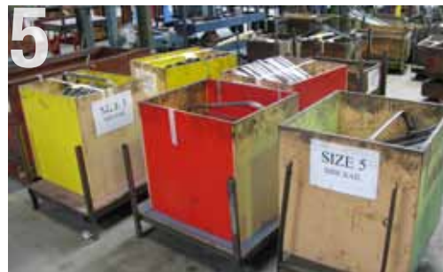
5 The welding bay – components stored in numbered and colour coded batches.
