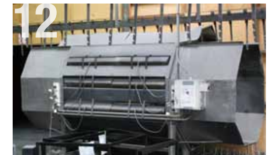
12 After powder coating the units are baked in the paint drier.
