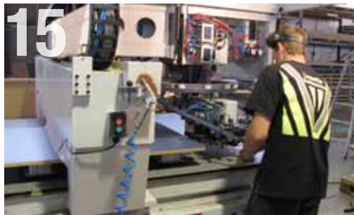
15 The cutting and drilling is done automatically by computer-controlled cutters on a large flat-bed machine.
