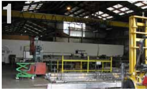
1 Steel is delivered to the steel storage bay, before it is cut, bent, welded, cleaned and powder coated.
