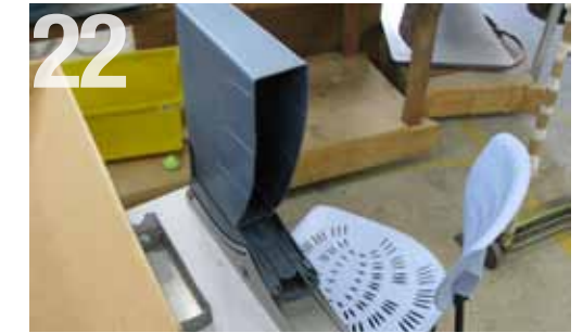
22 The main body is then fixed into the slider mechanism to complete the side storage unit.
