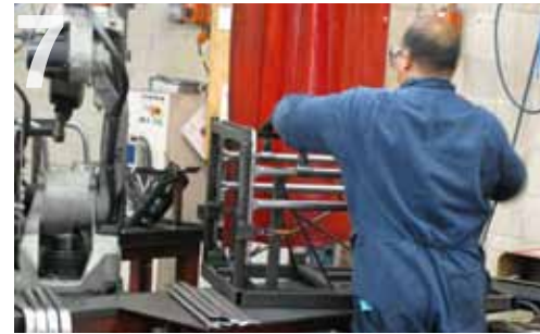
7 The pieces to be welded for a desk being set up in a jig. Pat: "Making a jig is quite an involved process, so if something changes it has to be really well thought through."
