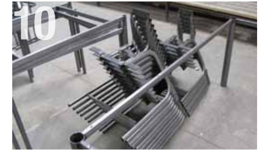
10 The cleaned units ready for powder coating.
